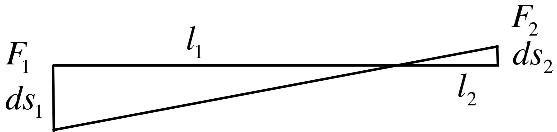
$$F_1 ds_1 = F_2 ds_2 \quad \frac{ds_1}{l_1} = \frac{ds_2}{l_2}$$
